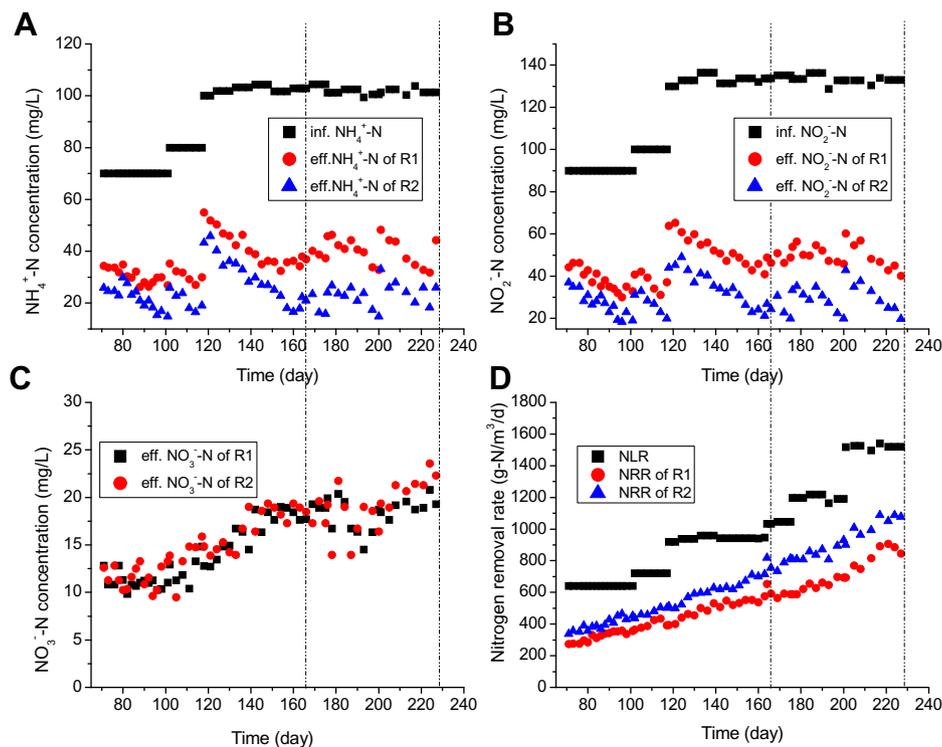
**Fig. 3.** Influent and effluent N concentration of each reactor during stable operation period. R1, control reactor; R2, reactor with 100 mg/L RGO addition. A, NH<sub>4</sub><sup>+</sup>-N; B, NO<sub>2</sub><sup>-</sup>-N; C, NO<sub>3</sub><sup>-</sup>-N; D, NLR and NRR. Nitrogen concentration increasing: day 70–165; HRT shortening: day 166–223.
