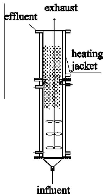
Fig. 1. Schematic diagram of the identical anammox reactor.
