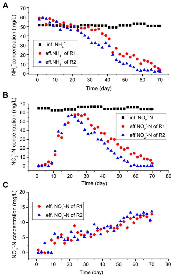
Fig. 2. Time course of influent and effluent N concentration of each reactor during start-up period. R1, control reactor; R2, reactor with 100 mg/L RGO addition. A,  $\text{NH}_4^+$ -N; B,  $\text{NO}_2^-$ -N; C,  $\text{NO}_3^-$ -N.
